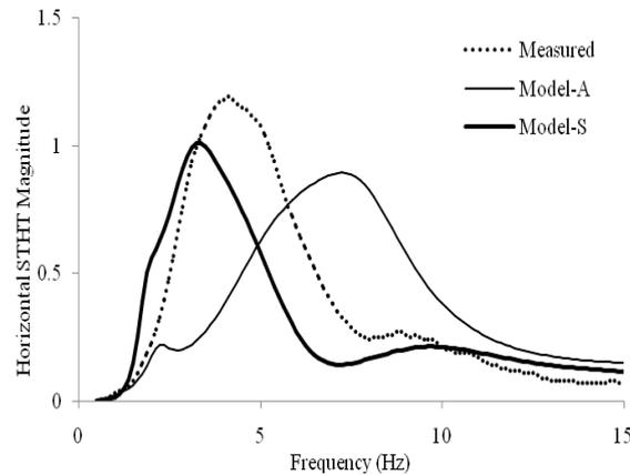
Figure 3: Comparison of horizontal STHT magnitude of Model-A and Model-S with the mean measured curve.
