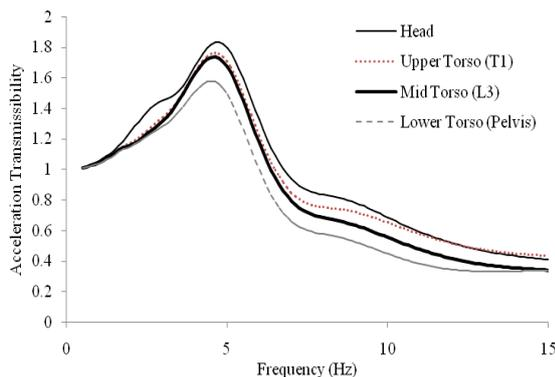
Figure 4: Vertical acceleration transmissibility magnitude between the seat and upper body segments of Model-S.
