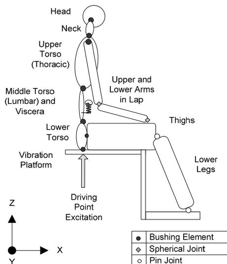
Figure 1: Sagittal plane view of the multi-body dynamic model of the body seated without a back support and exposed to vertical vibration from the seat.
