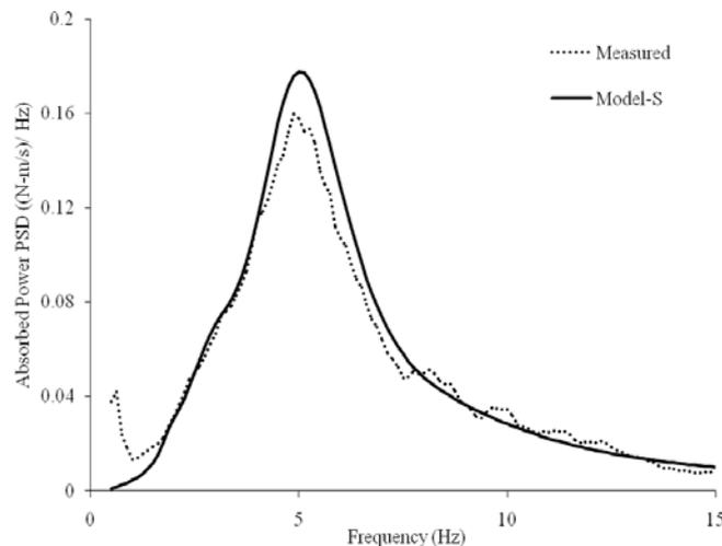
Figure 5: Spectral density of the Total Absorbed Power response of Model-S with the mean measured curve from 6 subjects evaluated at the driving point [22].
